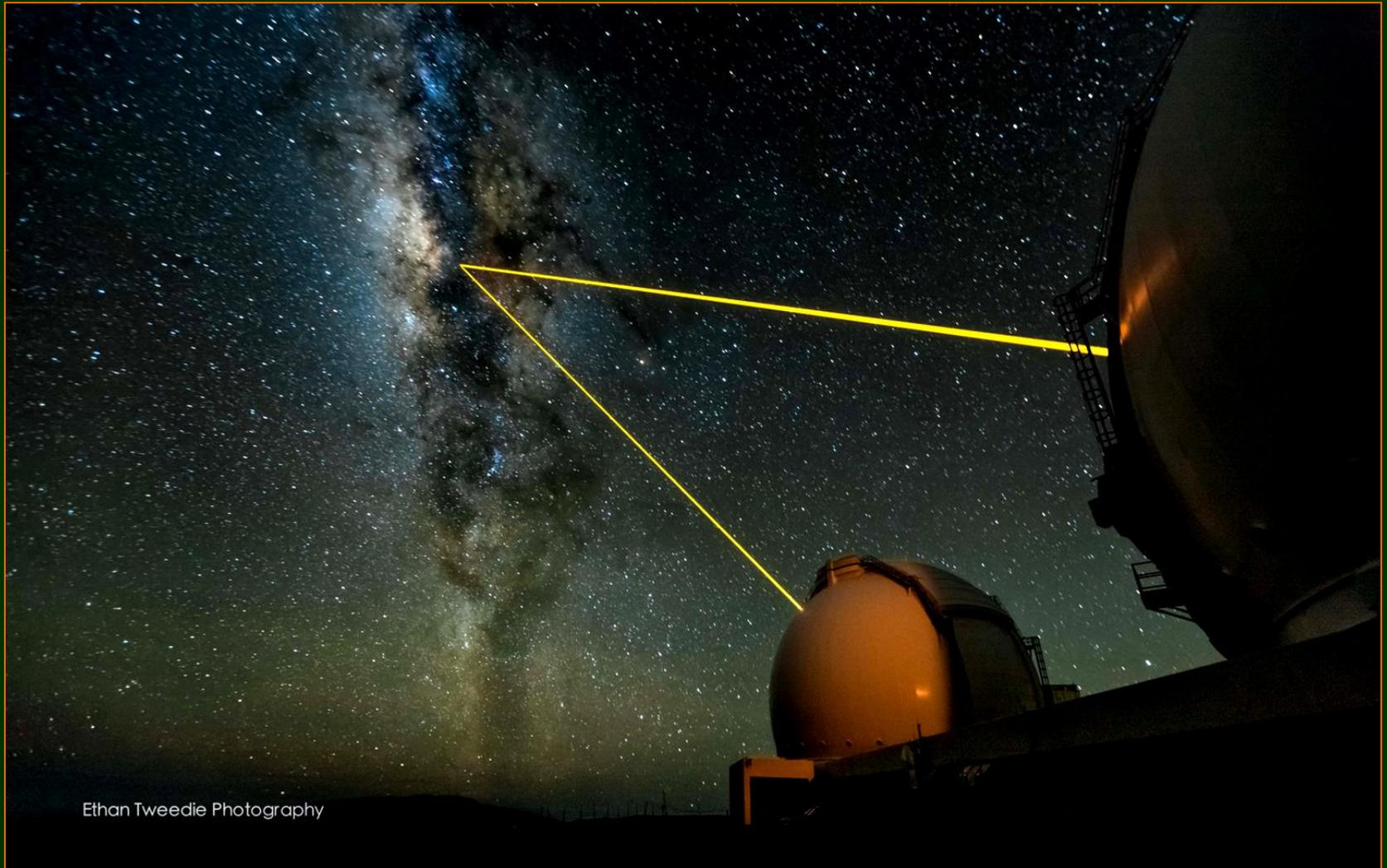
The two Keck Telescopes on Mauna Kea, Hawaii, observing the galactic center: The lasers are used to create an artificial star in Earth's upper atmosphere, which is then employed to measure the blurring effects of the lower atmosphere (that makes the stars twinkle in the night sky). The blurring gets corrected in real time with the help of a deformable mirror. This is the adaptive optics technique.
